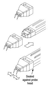
Use the variable spacing adapter to probe any two adjacent leads or test points spaced between 0.020 and 0.180-inches apart. Adjust the articulated pins by gently rotating them using a pair of tweezers.
